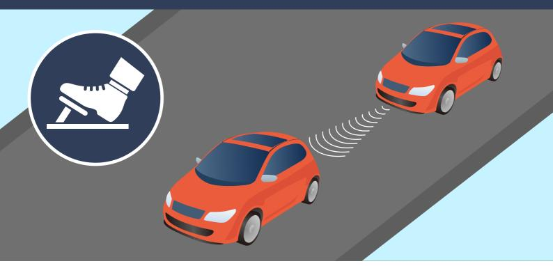
This relates to the inclusion of Advanced Driver Assistance Systems, otherwise known as ADAS. Cars can brake, steer and accelerate on behalf of the driver in certain situations. However, the human driver is still required to be in full control. Level 2 is the final layer of vehicle automation that needs the human to be fully monitoring all driving functions.
